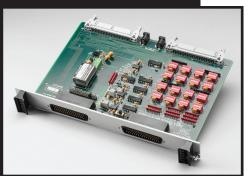
Keithley's EXP-1800 is a multiplexer/amplifier accessory for use with KPCI and DAS-1800 Series data acquisition boards. For thermocouple applications, the EXP-1800 offers cold junction compensation (CJC), open-TC detection, and low pass filtering. With a range of gain options, flexible packaging, and high performance, the EXP family offers a simple solution for a wide range of signal conditioning requirements.
